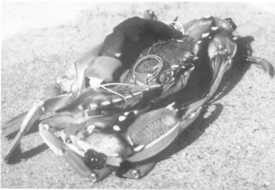
Fig. 1. Photograph of crab outfitted with a telemetry transmitter, showing preparation to monitor threat display activity (meral spread). On crab's chelae: reed-switches are secured to each dorsum of each merus, and magnets to each carpus
